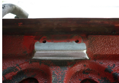
Figure 2. Dent repaired in boot-lid frame where lack of rear access required use of a “single-sided spot welder/dent puller”. Before and after. Black Magic?
