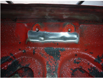
Figure 2. Dent repaired in boot-lid frame where lack of rear access required use of a “single-sided spot welder/dent puller”. Before and after. Black Magic?
