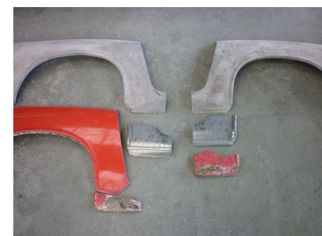
Figure 3. New panels used to provide templates to manufacture rust repair sections.
